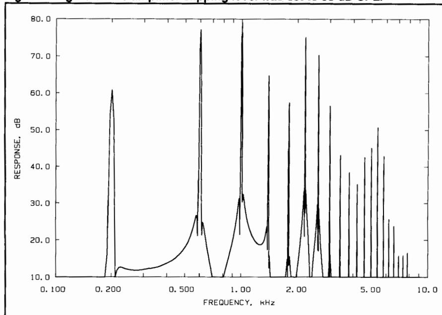
**Figure 3. Frequency response of a simulated two-channel hearing aid having a crossover frequency of 1500 Hz, gains of -20 dB in the low-frequency channel and 0 dB in the high-frequency channel, and an amplifier clipping level of 85 dB SPL. The response was measured with speech-shaped noise at a level of 70 dB SPL and smoothed using 1/3 octave bands.**
