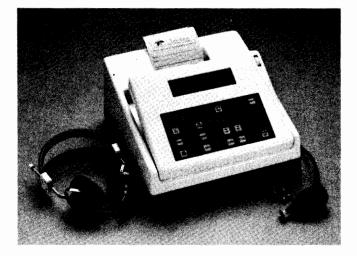
Teledyne Avionics, designer and manufacturer of high quality medical instrumentation, has introduced the TA-7B, an automatic impedance audiometer for school, pediatric and general medical practice hearing screening programs.
